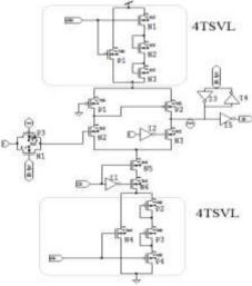
Fig 4. 4TSVL logic with SCCER
