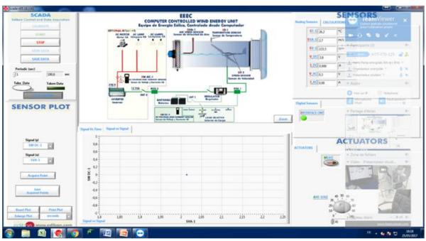
STEP 3 - Increase the fan speed so as to vary the speed of the area in the tunnel from minimum to maximum.
