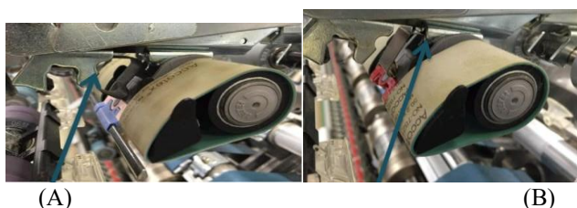
Fig.6. Old spring (A) and new spring (B).
