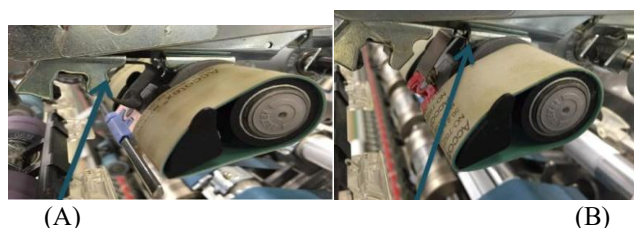
Fig.6. Old spring (A) and new spring (B).
