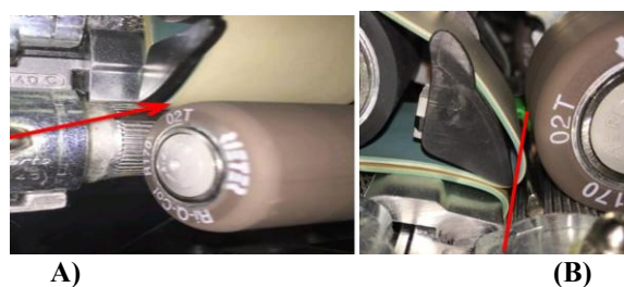
Fig.8. Correct setting of nose bar and cradle.
