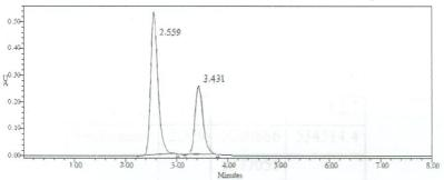
Figure 3: Chromatogram of the Standard mixture solution of Metformin hydrochloride and Atorvastatin calcium
