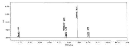
Figure 5: Chromatogram of Base Degradation
