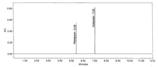
Figure 1: Chromatogram of Atazanavir and Cobicistat
