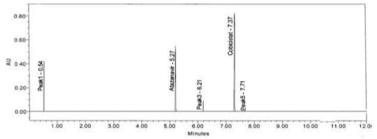
Figure 6: Chromatogram of Oxidative Degradation
