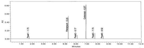
Figure 4: Chromatogram of Acid Degradation
