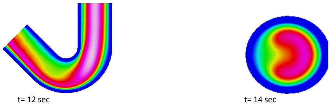
**fig.(5): velocity contours of the pipe's fluid for different time periods,  $Re=150$ , on a section along: (a) r-z plane , (b) r-θ plane**
