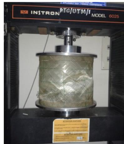
Fig.6b Buckled shell after test
