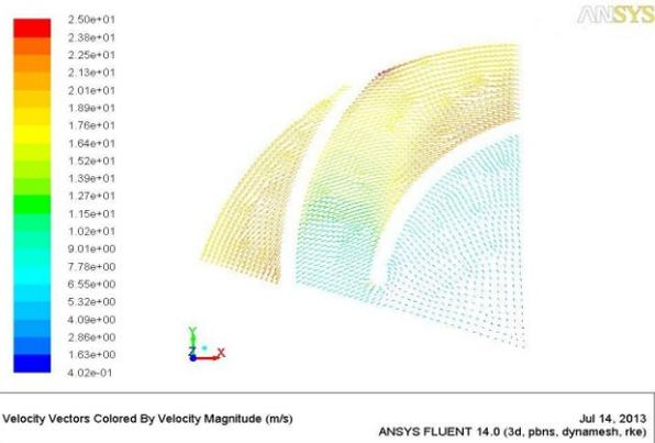
Figure(18) Velocity vectors in (X-Y)plane of hub at 2300rpm
