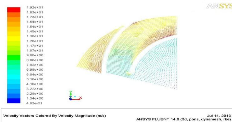
**Figure(6) Velocity vectors in (X-Y)plane of hub at 1900rpm**
