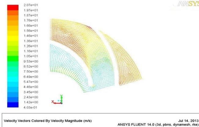
Figure(10) Velocity vectors in (X-Y)plane of shroud at 2000rpm
