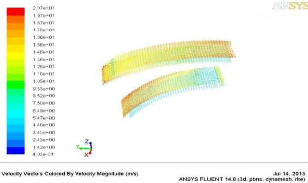
Figure(8) Velocity vectors in (Z-Y)plane of blade at 2000rpm
