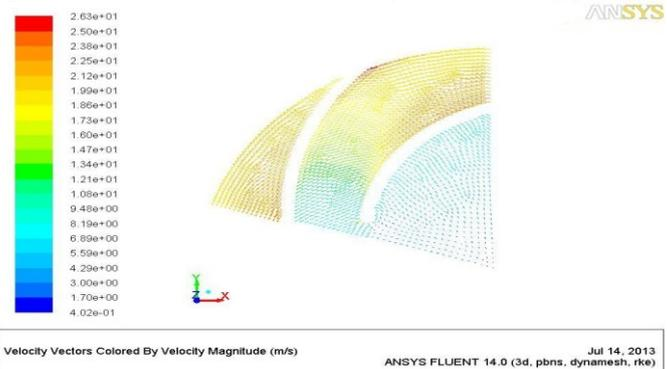
Figure(21) Velocity vectors in (X-Y)plane of hub at 2400rpm
