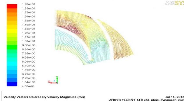
**Figure(7) Velocity vectors in (X-Y)plane of shroud at 1900rpm**
