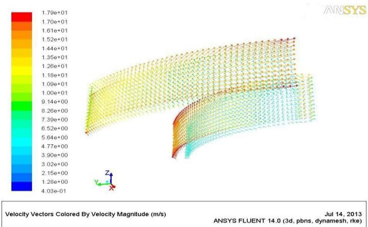
Figure(2) Velocity vectors in (Z-Y)plane of blade at 1800rpm
