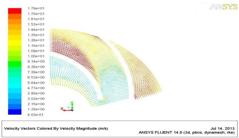
Figure(4) Velocity vectors contours in (X-Y)plane of shroud at 1800rpm
