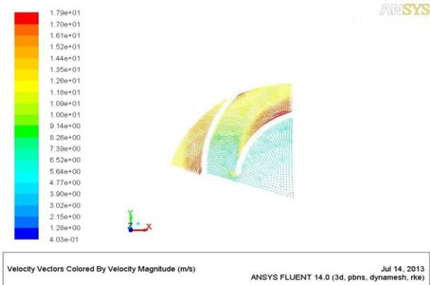
Figure(3) Velocity vectors in (X-Y)plane of hub at 1800rpm
