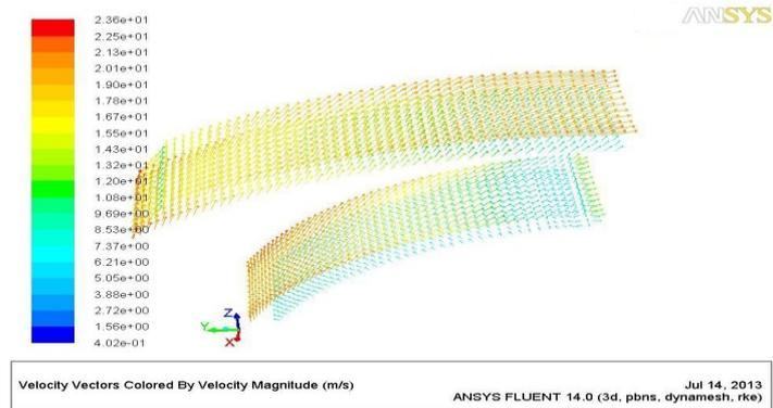
Figure(14) Velocity vectors in (Z-Y)plane of blade at 2200rpm
