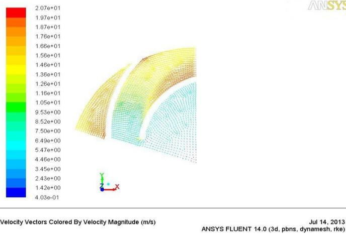
Figure(9) Velocity vectors in (X-Y)plane of hub at 2000rpm
