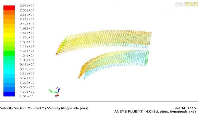
Figure(20) Velocity vectors in (Z-Y)plane of blade at 2400rpm
