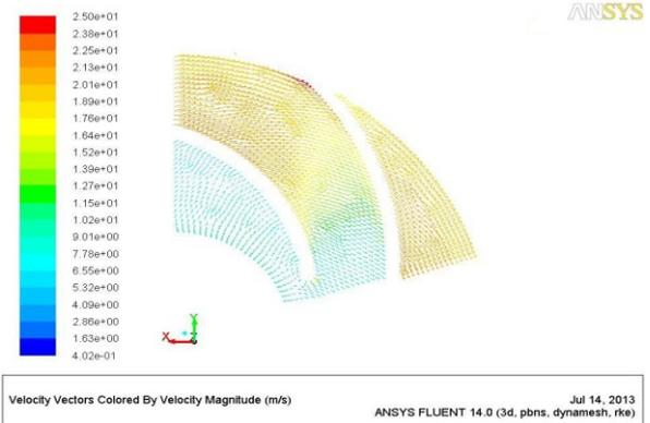
Figure(19) Velocity vectors in (X-Y)plane of shroud at 2300rpm
