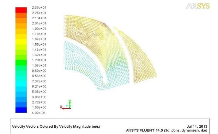
Figure(13) Velocity vectors in (X-Y)plane of shroud at 2100rpm
