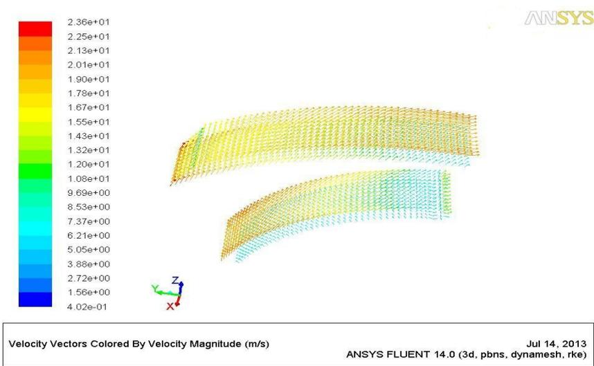
Figure(11) Velocity vectors in (Z-Y)plane of blade at 2100rpm
