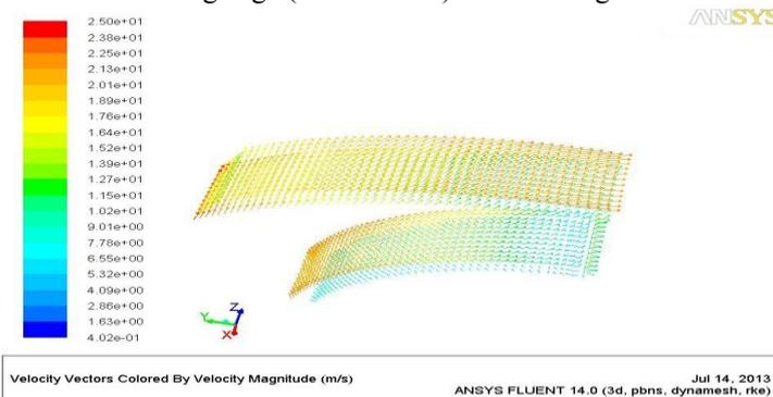
Figure(17) Velocity vectors in (Z-Y)plane of blade at 2300rpm
