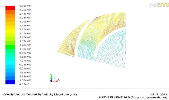
Figure(12) Velocity vectors in (X-Y)plane of hub at 2100rpm
