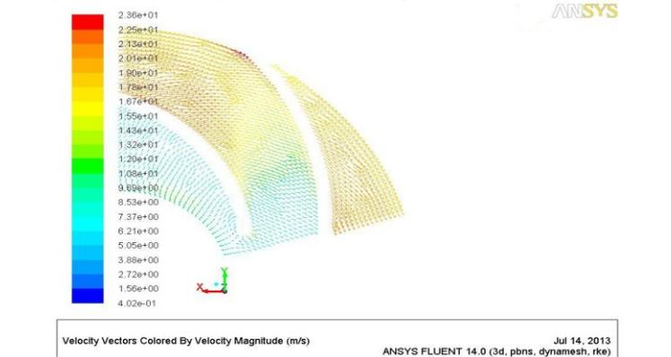
Figure(16) Velocity vectors in (X-Y)plane of shroud at 2200rpm
