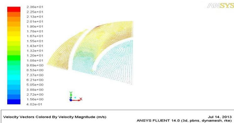
Figure(15) Velocity vectors in (X-Y)plane of hub at 2200rpm
