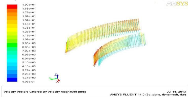
**Figure(5) Velocity vectors in (Z-Y)plane of blade at 1900rpm**
