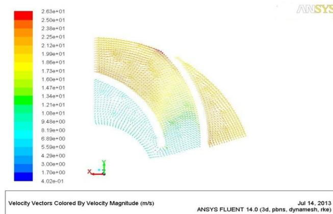
Figure(22) Velocity vectors in (X-Y)plane of shroud at 2400rpm
