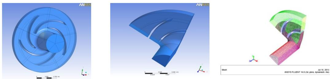
(a) Centrifugal pump geometry (b) Single blade passage geometry and mesh
