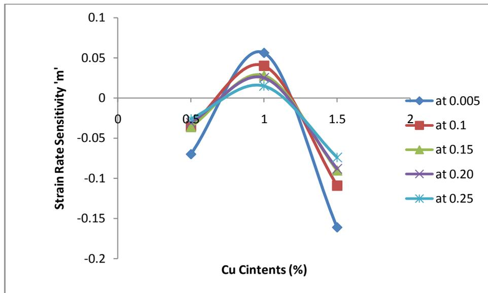
Fig. 30 Strain Rate Sensitivity 'm' v/s Cu Contents
