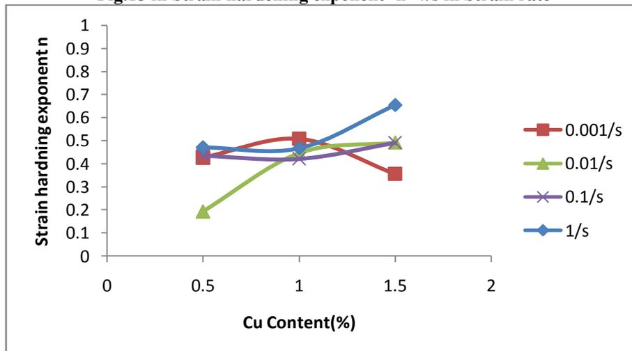
Fig.16 Strain hardening exponent 'n' v/s Cu content
