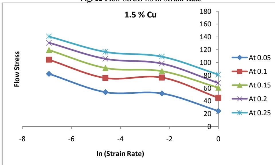
Fig 23 Flow Stress v/s ln (Strain Rate)
