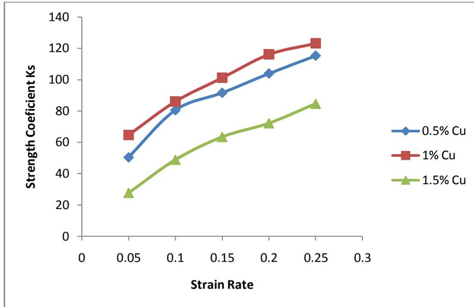
Fig. 27 Strength Coefficient 'Ks' v/s Strain Rate
