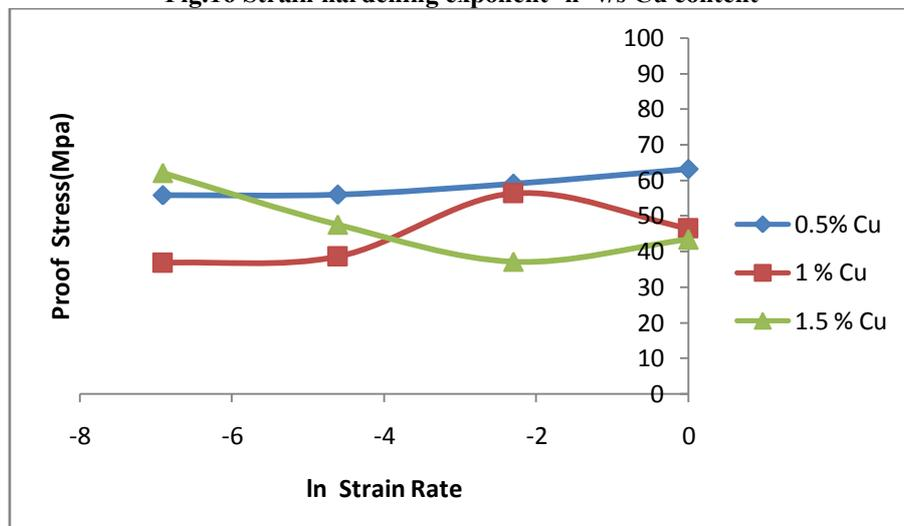
Fig.17 Proof Stress v/s ln Strain rate
