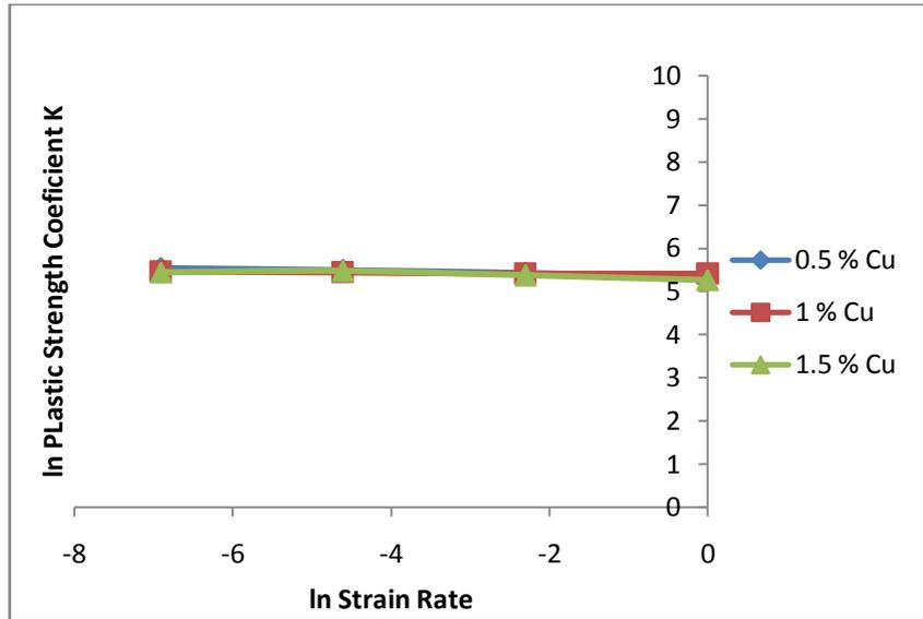
Fig. 12 ln Plastic Strength coefficient 'k' v/s ln Strain rate
