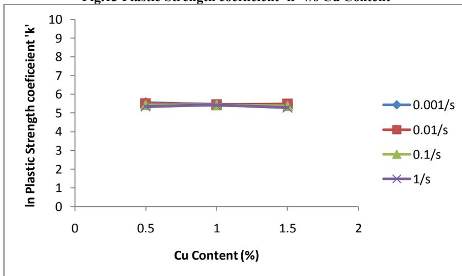
Fig. 14 ln Plastic Strength Coefficient 'k' v/s Cu Content
