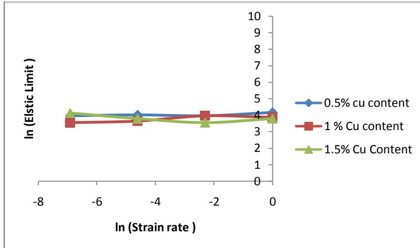
Fig.9 ln Elastic limit v/s ln Strain rate
