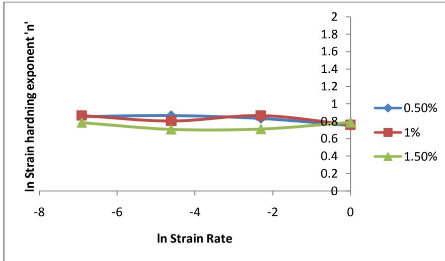
Fig.15 ln Strain hardening exponent 'n' v/s ln Strain rate
