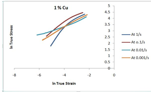
Fig 5 In True Stress v/s In True Strain
