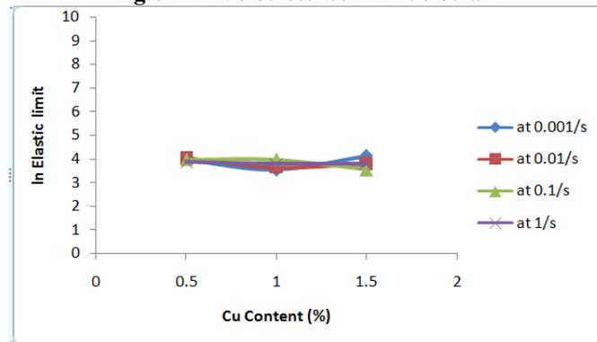
Fig 7 In Elastic limit v/s Cu Contents
