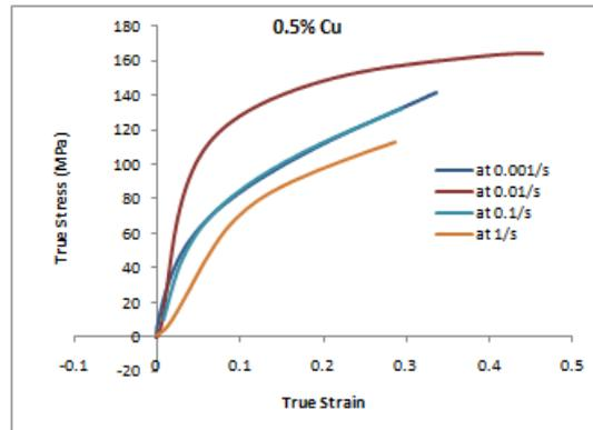
Fig 1 True Stress V/S True Strain (0.5% Cu)
