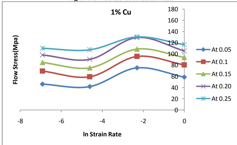
Fig. 22 Flow Stress v/s ln Strain Rate
