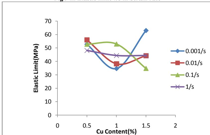
Fig.10 Elastic limit v/s Cu contents
