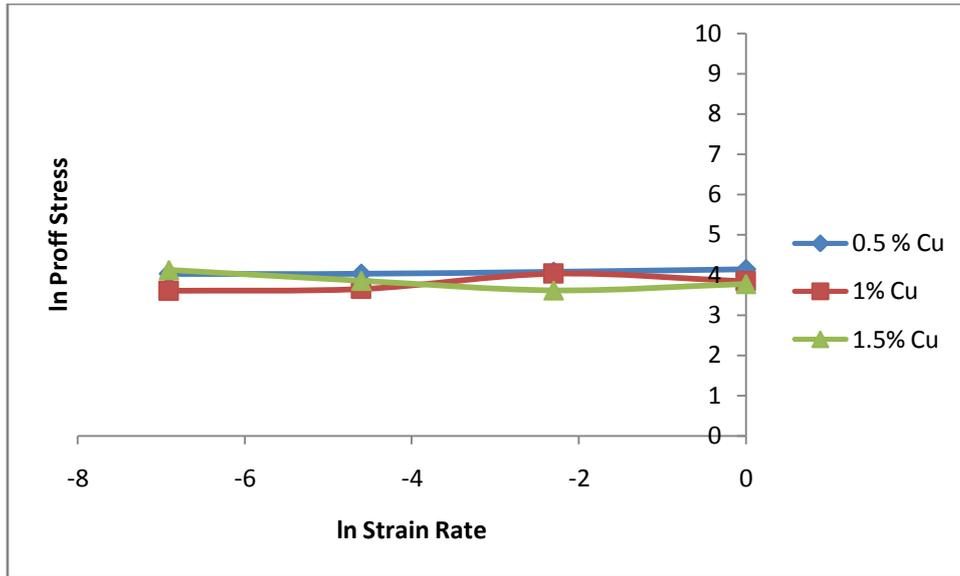
Fig.18 ln Proof Stress v/s ln Strain arte
