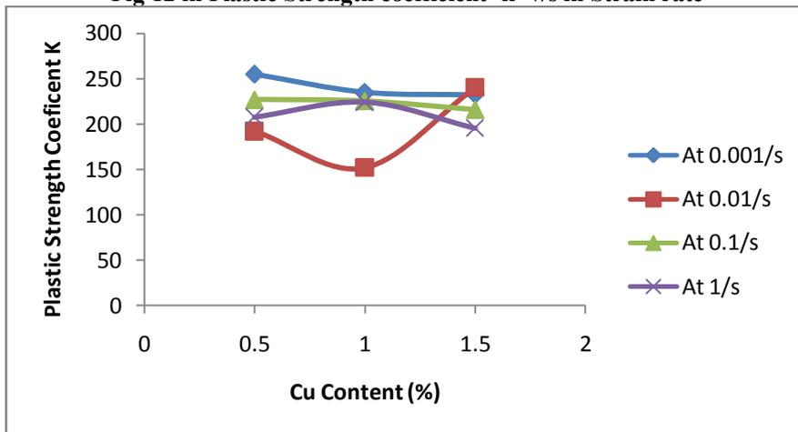
Fig.13 Plastic Strength coefficient 'k' v/s Cu Content
