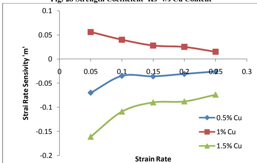
Fig.29 Strain Rate sensitivity 'm' v/s Strain Rate
