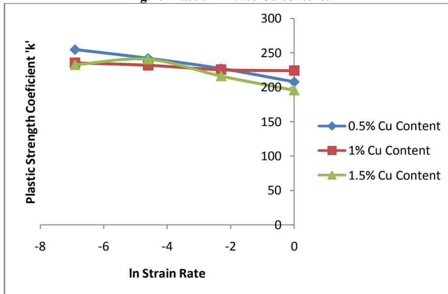
Fig.11 Plastic strength coefficient 'k' v/s ln Strain rate
