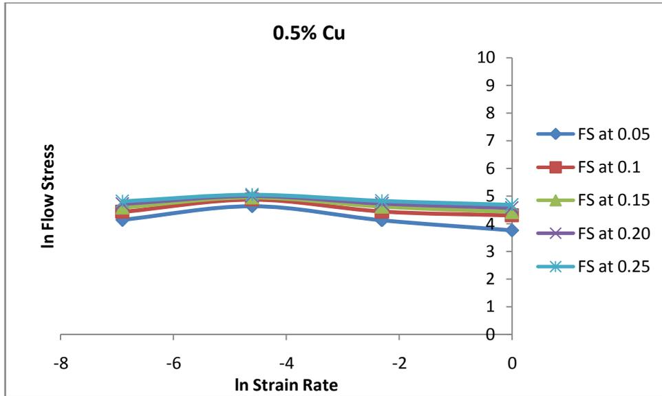
Fig. 24 In Flow Stress v/s In Strain Rate
