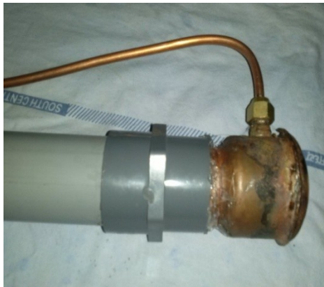
Figure: Inlet portion of Helium gas with valve
