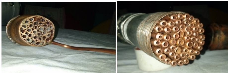
Figure 16. Copper tubes arranged parallel to the wave propagation
