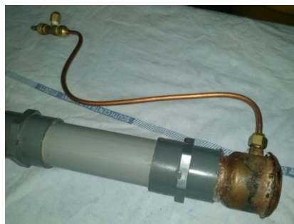
Figure: Copper pipe arrangement projected outside for gas filling and evacuating provided by a valve
