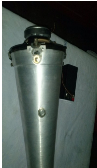
Figure: A conical section for intensifying of sound wave
