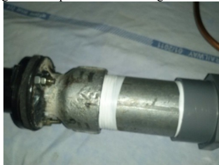
Figure: Hot heat exchanger sealed with glue and Teflon tape.
