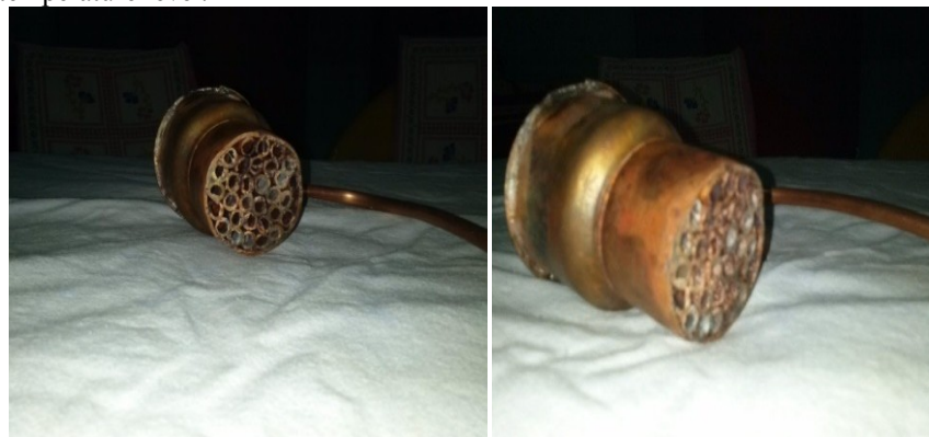
Figure 12. Copper tubes of cold side of stack which function as cold heat exchanger other end is closed by a copper cap.
