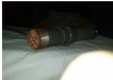
Figure 14. Copper tubes with iron sleeve attached to hot side of stack
