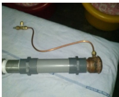
Figure 18. Hot and cold heat exchangers are thermally separated by PVC pipe.
