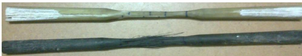
**Figure 7:** Tensile Tested Samples (Glass/Epoxy, Carbon/Epoxy)
