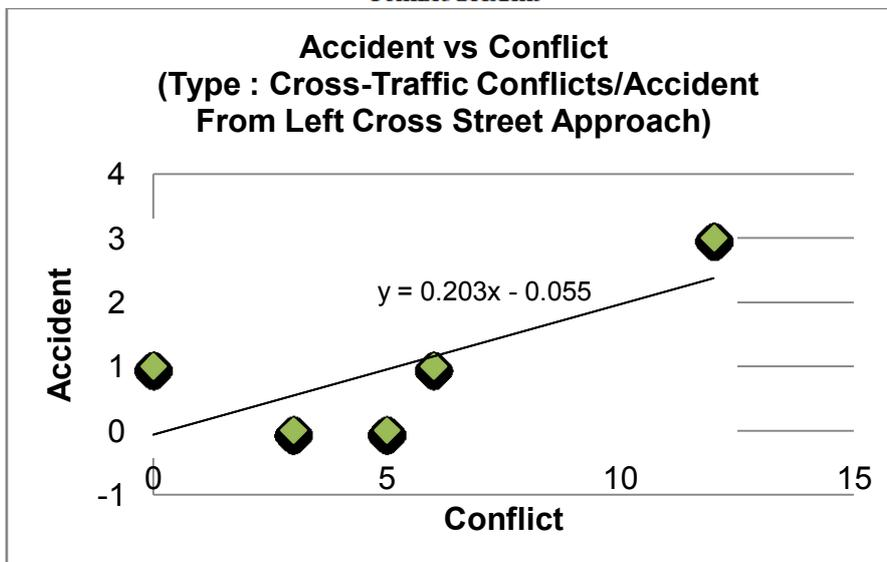
Figure 4.5: Relationship between accident and conflict for cross traffic/accident From left cross street approach
