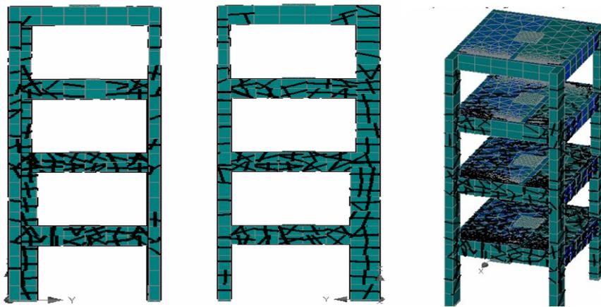
Figure 12. Crack Patterns at Step-344 at Base-Shear-962KN
