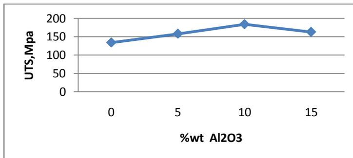
**Fig: 3.1.1** Variation of UTS with % wt variation of Al<sub>2</sub>O<sub>3</sub>
