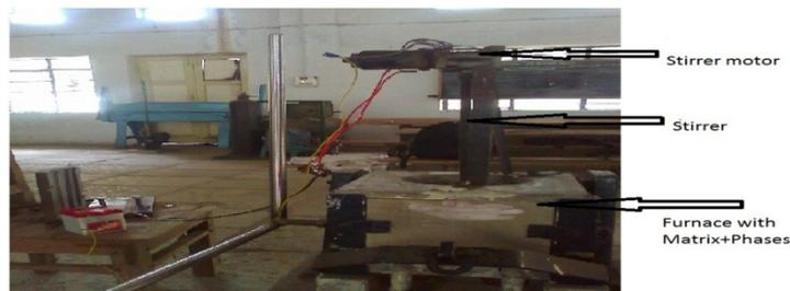
**Fig 2.1.3 Induction furnace with stirrer mechanism**
