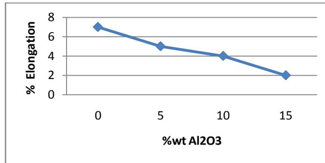
Fig:3.3.1 Variation of % Elongation with % wt Al<sub>2</sub>O<sub>3</sub>
