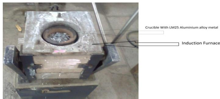
**Fig.2.1.1 Induction furnace with Crucible containing LM25**
