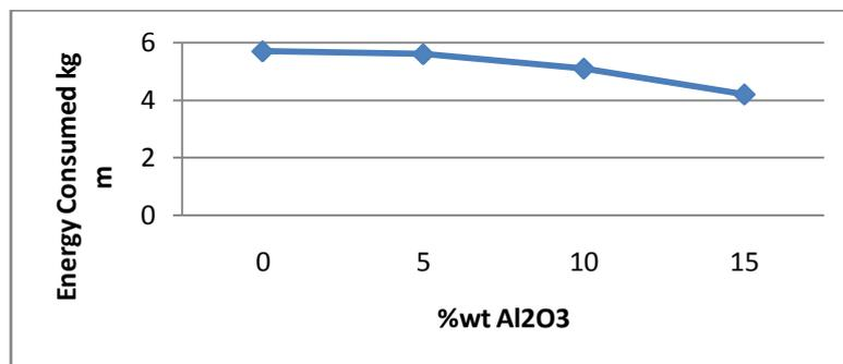
Fig:3.4.1 Impact load absorption(In kg m) with % wt Al<sub>2</sub>O<sub>3</sub>
