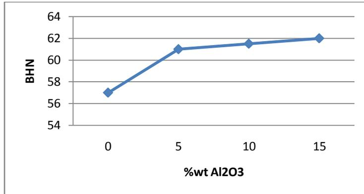
Fig:3.2.1 Hardness variation With % wt variation of AL<sub>2</sub>O<sub>3</sub>.
