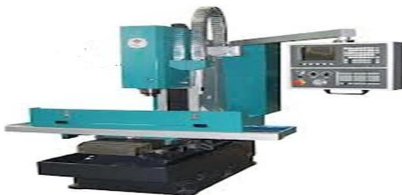
**FIG 1.3 CNC Milling Machine**
