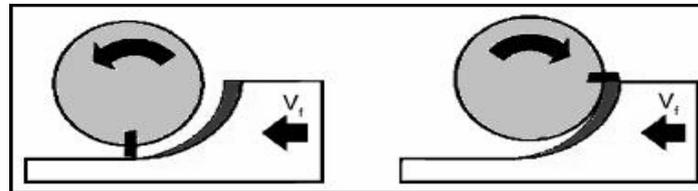
Fig. 2.1 Up milling and down milling process
