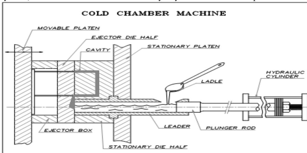
Fig. 1.2 Cold-Chamber Machine
