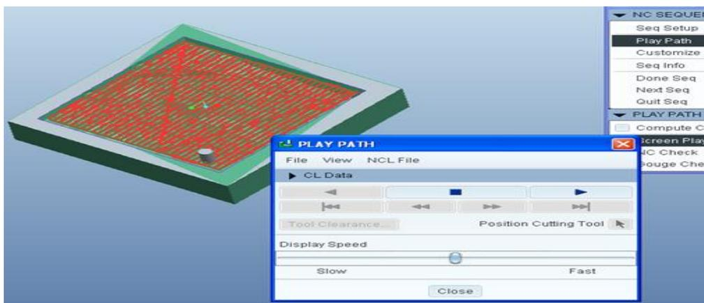
After completion of tool play path to check the required part shape is obtained or not checked by using NC check in Pro/E. It is illustrated in fig.2.6
