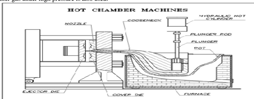
Fig. 1.1 Hot-Chamber Machine
