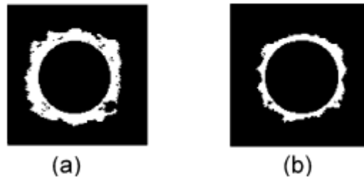
Figure 2.1: Ultrasonic C-Scan showing the extent of drilling-induced delamination for different drills (feed rate, 0.01 mm/rev; spindle speed, 1000 rpm; drill diameter, 8 mm). (a) twist drill (b) candle stick drill (c) saw drill. [2] Delamination factor with ultrasonic C-Scan is shown in figure 2.2. They resulted as feed rate and drill diameter are seen to make the largest contribution to the overall performance and the candle stick drill and saw drill cause a smaller delamination factor than twist drill.
