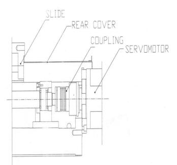
Figure6. Ball Screw Arrangement
