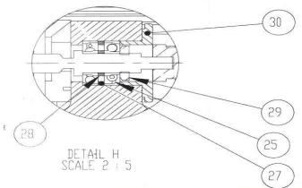
Figure2. Ball Screw Sectional View
