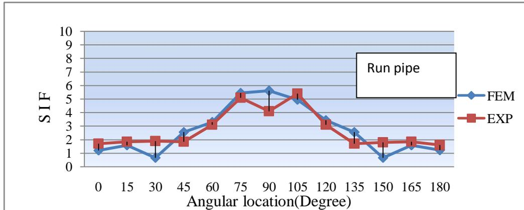
Fig. No. 6 Intersection stresses-run pipe moment (run pipe),  $M_{xr}$
