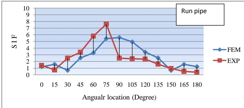
Fig No. 10 Intersection stresses-run pipe moment (run pipe), $M_{xb}$
