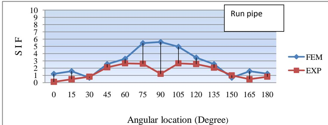
Fig No. 8. Intersection stresses-run pipe moment (run pipe), $M_{yr}$
