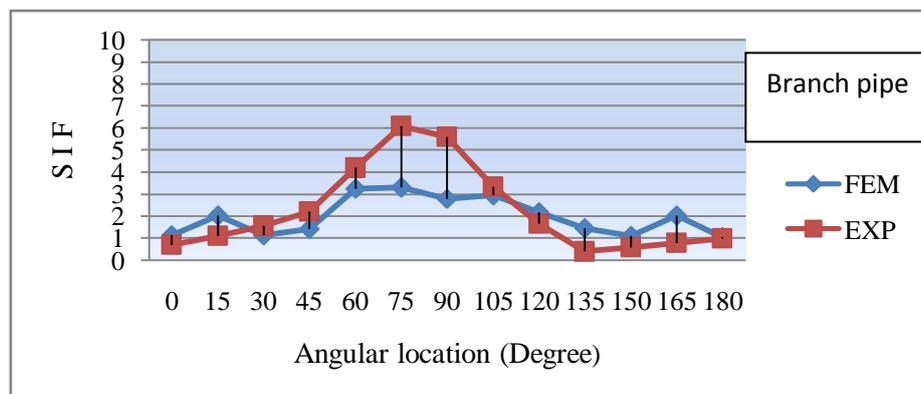
Fig No. 11 Intersection stresses-run pipe moment (branch pipe), $M_{xb}$
