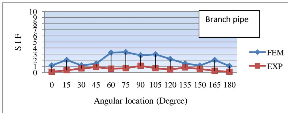
Fig No.9 Intersection stresses-run pipe moment (branch pipe), $M_{yr}$
