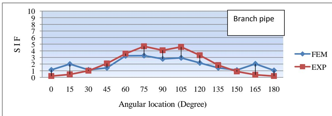
Fig No. 7 Intersection stresses-run pipe moment (branch pipe),  $M_{xr}$
