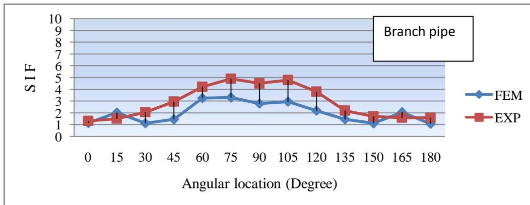
Fig No. 13 Intersection stresses-branch pipe moment (branch pipe), $M_{yb}$
