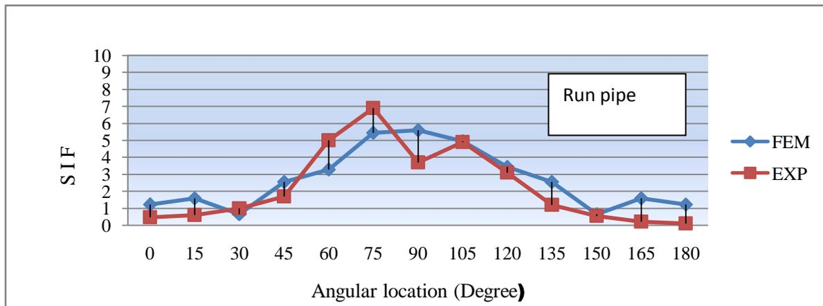
Fig No. 12 Intersection stresses-branch pipe moment (run pipe), $M_{yb}$
