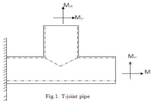
It is evident from the geometry of T-joint pipe shown in fig.1; there is change in geometry at the intersecting junction which leads to stress concentration effect at the intersecting junction. Due to this, probability of failure increases at this location. In this work an effort is made to study the stress intensity at intersecting junction of run and branch pipe. T pipe joint is considered for stress analysis. The loading under internal pressure and moments is considered.
