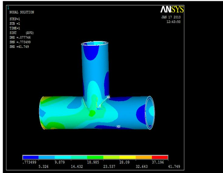
Fig.5. Stress intensity of T-joint pipe
