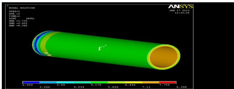
Fig.no.4 Stress intensity of plane pipe
