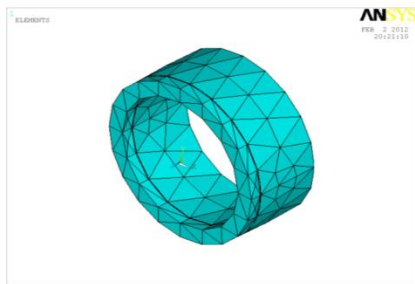
Fig. 2.1: 3-Dimensional Model Meshing
