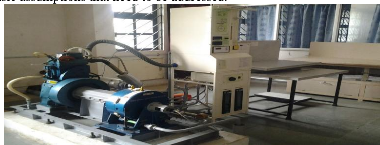
Fig 2.3: Figure showing single cylinder, four stroke, and VCR (Variable Compression Ratio) Diesel engine
