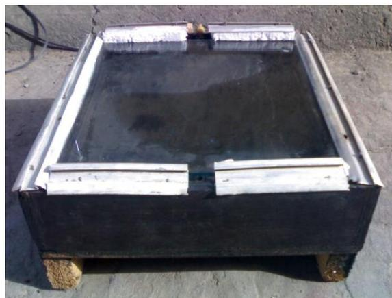
Fig. 2: Actual view of Direct absorption solar collector
