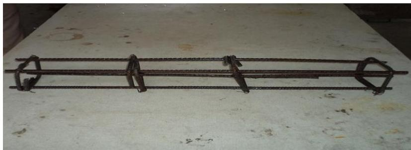
Figure-II Conventional RTS Bar fabrication
