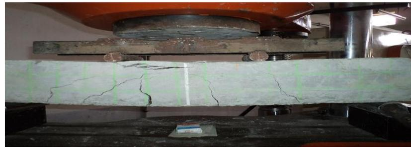
Figure-V Failure of DSSR Beam-2
