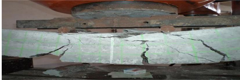
Figure-IV Failure of DSSR Beam-1
