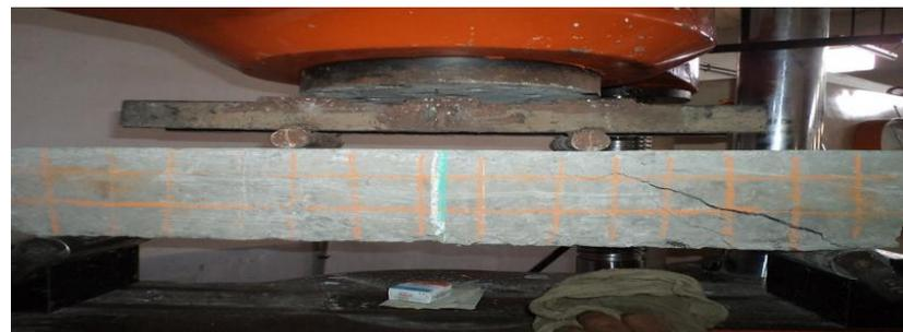
Figure-VI Failure of RTSR Beam-2
