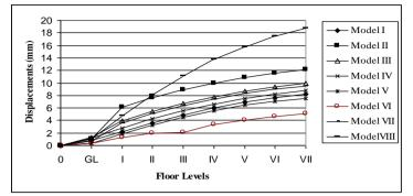
Figure 1: Displacement Profile in Longitudinal Direction for Zone IV (ESA)
