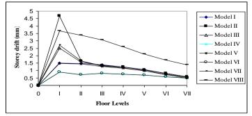
Figure 3: Storey Drift Profile in Transverse Direction for Zone IV (ESA)
