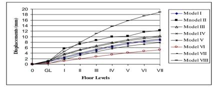
Figure 2: Displacement Profile in Transverse Direction For Zone IV (ESA)
