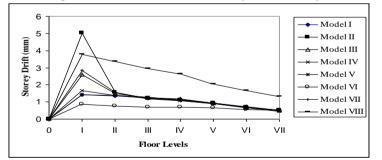
Figure 2: Storey Drift Profile in Longitudinal Direction for Zone IV (ESA)
