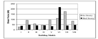
Figure 7: Comparison of Maximum Shear Force in Transverse Direction for Zone IV (ESA)
