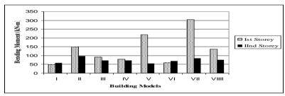
Figure 5: Comparison of Maximum Bending Moment in Transverse Direction for Zone IV (ESA) The maximum shear forces in the columns in longitudinal and transverse direction are shown in Figure 6 and Figure 7.
