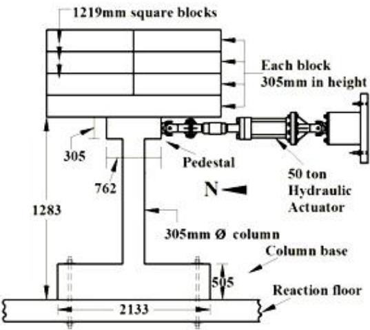
Fig. 2: Side view (Elevation) of the test bridge column
