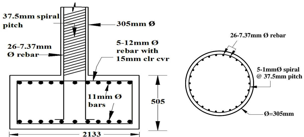
Fig.3: Reinforcement details of bridge column
