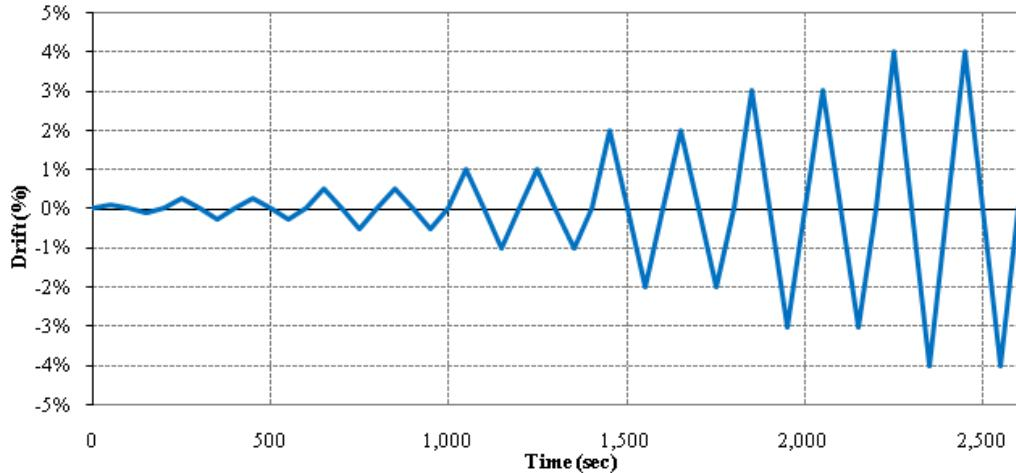
*Fig.5: Loading protocol used for testing the columns*
