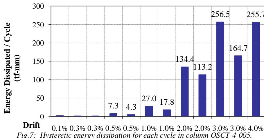
Fig.7: Hysteretic energy dissipation for each cycle in column QSCT-4-005.
