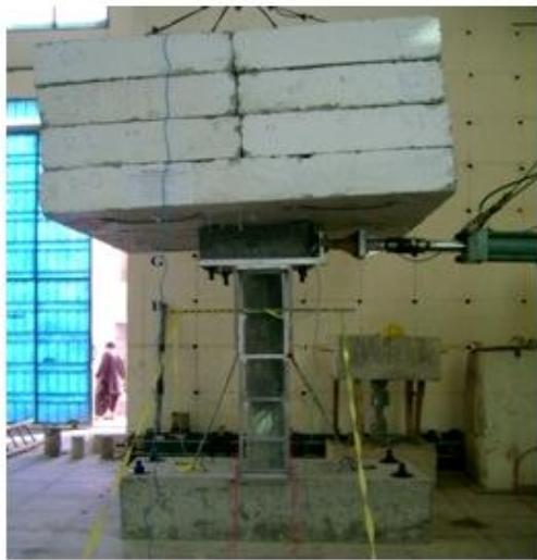
Fig. 1. Scaled RC bridge columns
