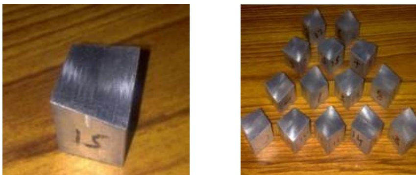
Fig 2.4: CNC milled freeform surface
