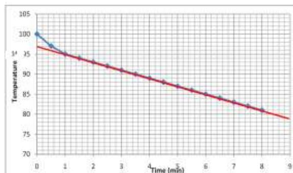
Fig 2: Temperature vs. Time for Borosilicate glass during cooling
