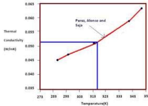
Fig 7: Experimental thermal conductivity as a function of the temperature, Alveolit samples of insulation foam.
