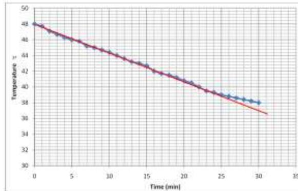
Fig 4: Temperature vs. Time for polyolefin foam faced aluminum foil during cooling.
