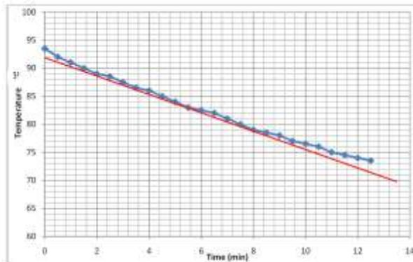
Fig 3: Temperature vs. Time for Styrene Butadiene Rubber during cooling
