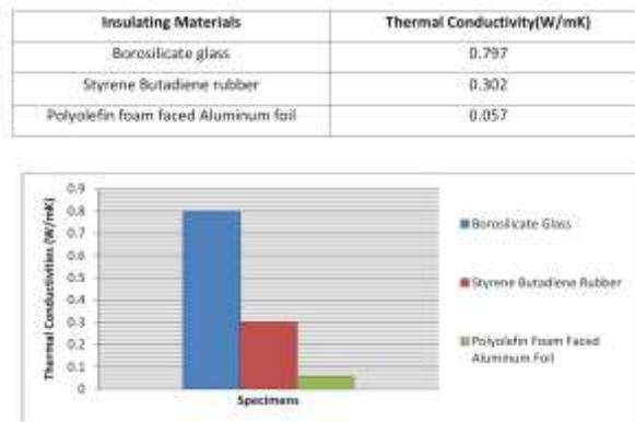
Figure 8: Comparison of thermal conductivity of Borosilicate glass, Styrene Butadiene rubber and Polyolefin foam faced Aluminum foil.
