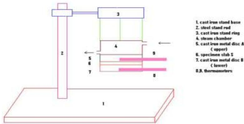
Figure 1: Schematic view of Lee's and Charlton's Apparatus
