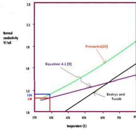
Fig 5: Determined True thermal conductivities of glass with variation on Temperature.
