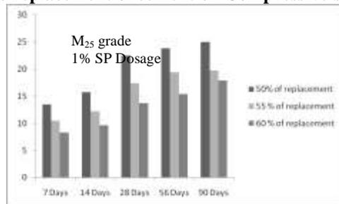
Fig.6 Effect of age and % replacement of cement on Compressive strength for 1% SP Dosage
