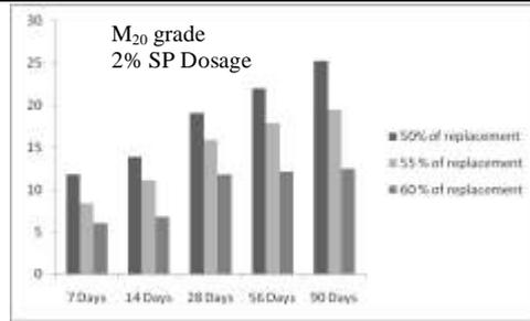
Fig.4 Effect of age and % replacement of cement on Compressive strength for 2% SP Dosage
