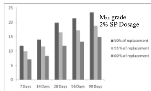
Fig.8 Effect of age and % replacement of cement on Compressive strength for 2% SP Dosage
