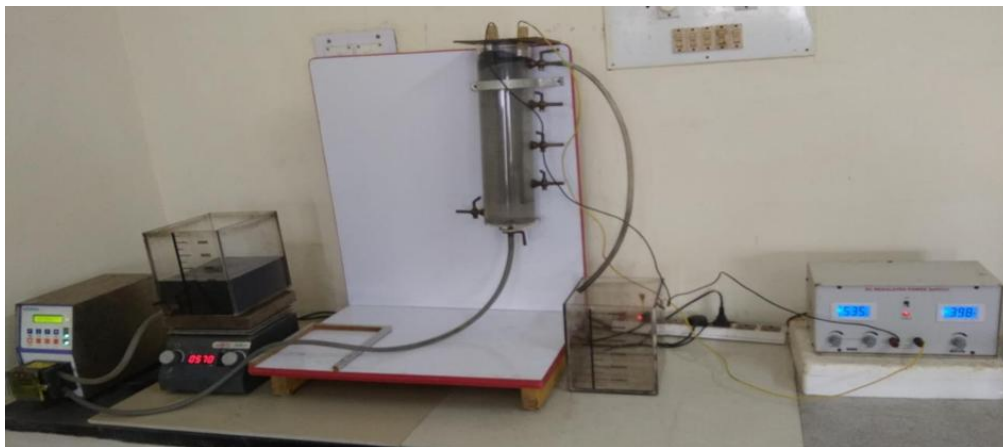
Figure 1 Experimental set-up of Continuous electrocoagulation
