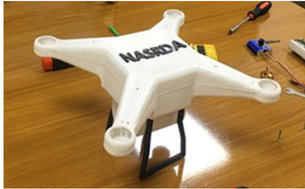
Fig 20: Final Frame Produced by Rapid Prototyping
