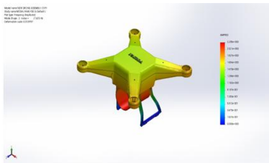
Fig 16: Amplitude Plot for Mode Shape 3 (Value = 27.6346 Hz) Min: 0, Max: 2.20499
