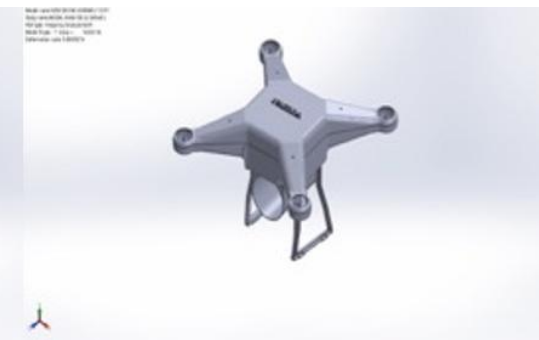
Fig 18: Amplitude Plot for Mode Shape 5 (Value = 102.139 Hz) Min: 0, Max: 4.26937
