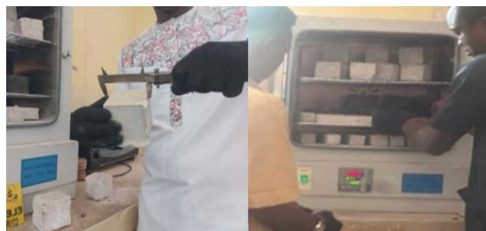
Plate 4: Concrete samples subjected to 150°C elevated temperature for 6 hours
