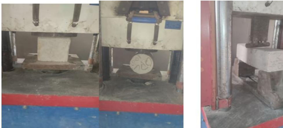
Plate 3: (a) Cube (b) Cylinder and (c) Flexural beam under UTM test
