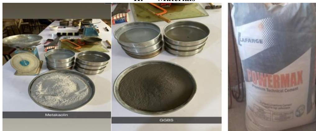
Plate 1: (a) metakaolin, (b) GGBFS and (c) LPcem
