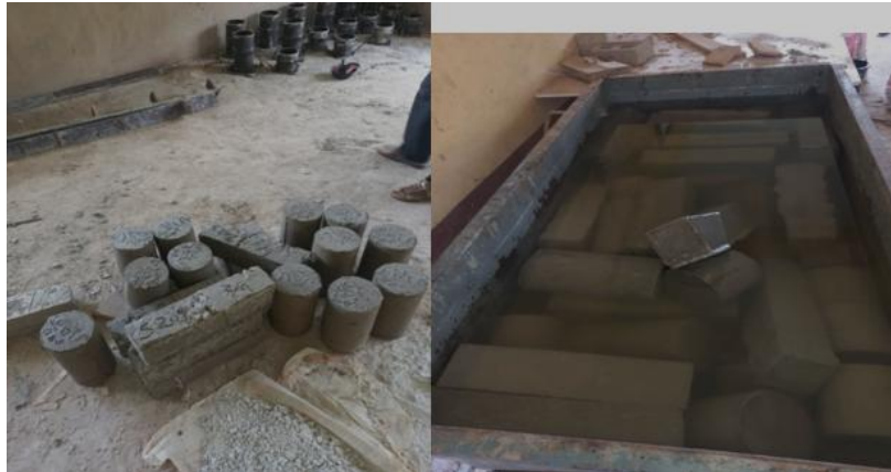
Plate 2: (a) Cast (b) cured samples respectively
