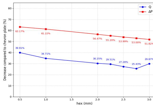
Fig.6: Decrease in heat transfer rate and pressure drop in cylindrical extrusion plate compared to chevron plate
