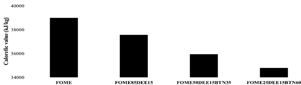
Fig. 5 Calorific values of FOME and its blends
