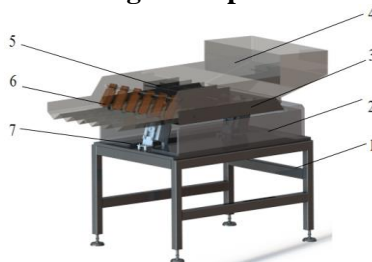
Fig.1 Overall structure of the vibration feeding device
