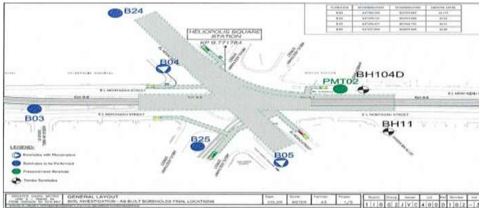
Figure 3 Locations of Borehole at Heliopolis Underground Station
