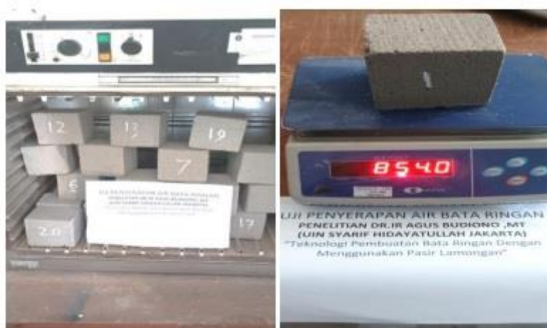
Figure 1. Test Sample and weighing of weight and water absorption testing of light brick
