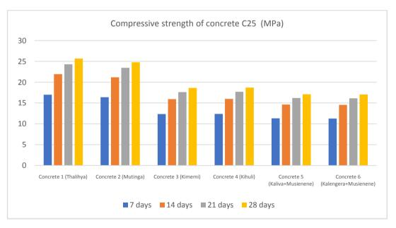
Figure 6. Concrete compression strength C25
