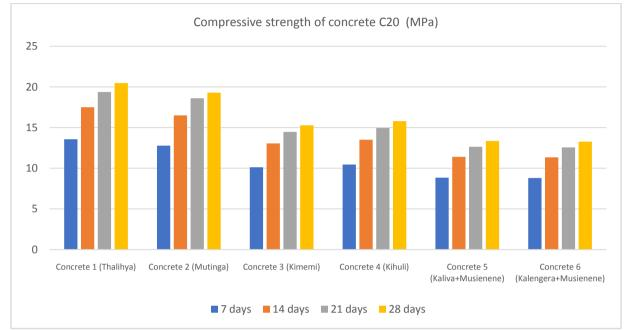
Figure 5. Concrete compression strength C20
