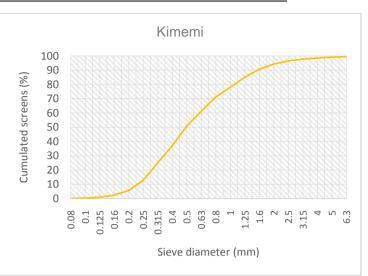
Figure d. Particle size curve of Kimemi sand
