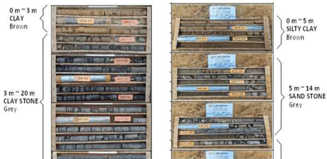
Figure 5. Borlog of Clay Shale At the Nation's Capital (IKN)
