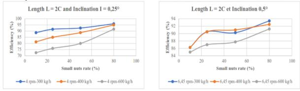
a: Efficiency for 2C length and 0,25° inclination Figure 3: Efficiency of calibrator for a short drum
