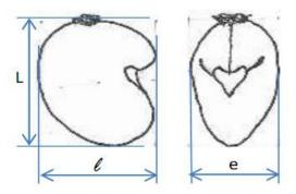
Figure 1: Main dimensions of a cashew raw nut: L = Length; *l*=width; e= thickness
