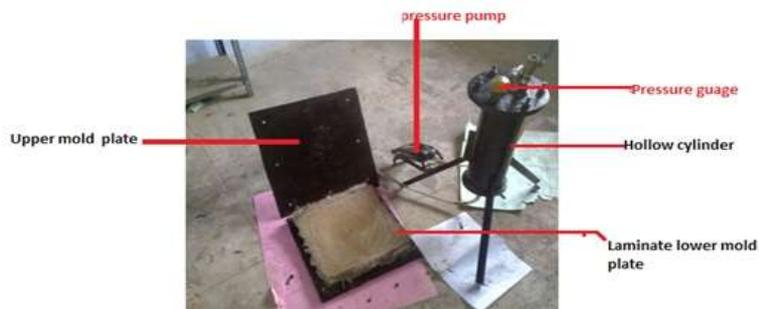
Fig1:RTM with Composite laminate piece
