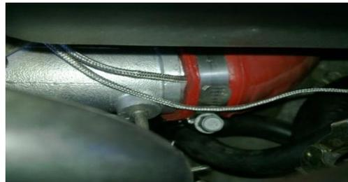
Picture4- thermistor fitted at the inlet of intercooler
