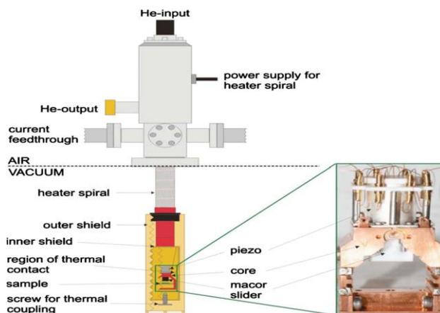
Fig: 3.1 Low Temperature-AFM and the flow cryostat
