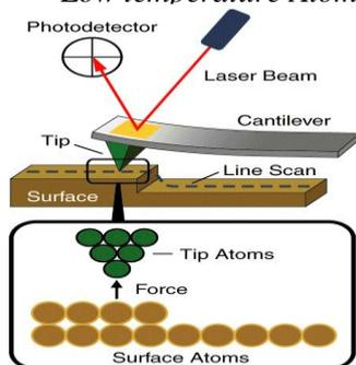
Fig:1 Principal Of Atomic Force Microscope
