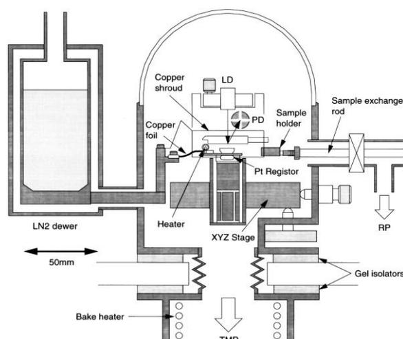
**Fig. 3.3 Cross sectional drawing of the AFM.**
