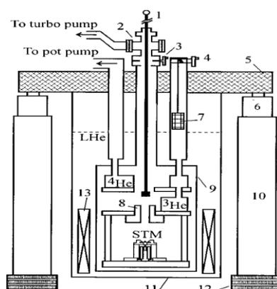
Fig: 3.2 STM Cryostat And Vibration-Isolation.
