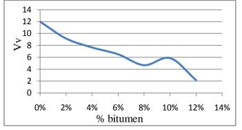
Fig 4.2.4: Relation between voids ratio (Vv) and bitumen content
