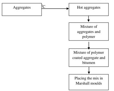
Fig 3.3: Waste Plastics Blended With Bitumen - Aggregate Mix- Process (Dry)
