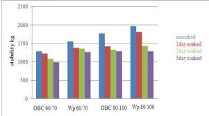
Fig 4.5.1: Comparison of soaked and unsoaked test results
