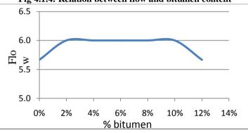
Fig 4.1.4: Relation between flow and bitumen content
