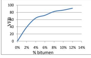
Fig 4.1.3: Relation between voids filled with bitumen (VFB) and bitumen content
