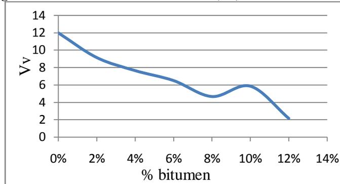
**Fig 4.2.5: Relation between flow and bitumen content**
