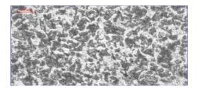
Fig 6(b) 200X Nital Core structure after Quenching.
