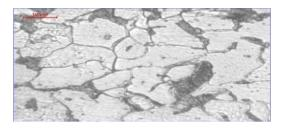
Fig 6(c) 500X Nital Core structure before quenching.
