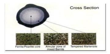
Fig.5: Shows the microstructure at surface and core.
