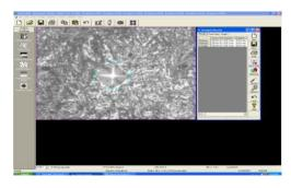
Fig 7(b) 500X Nital.MicroHardnesss 300 ~ 320Hv,After Quenching.
