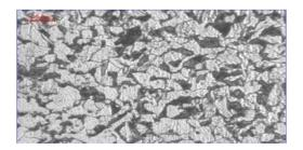
Fig 6(a) 200X Nital Core structure before Quenching.
