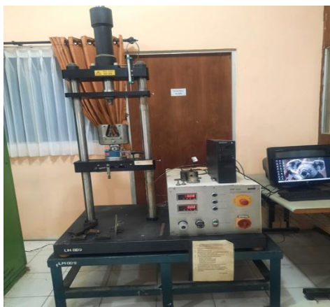
Figure 2. Tensile Testing Equipment Model WP 310 Gunt Hamburg Material Testing Machine
