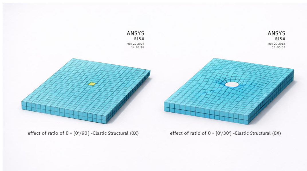
Figure 2: Model of square plate without and with cut-out
