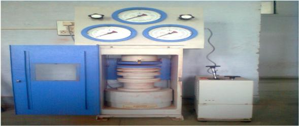
Figure 1 Compressive Strength Testing Machine
