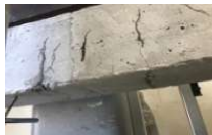
Fig. 2. Stages of repairing RC beams using epoxy injection technique (continued)
