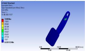
The value of total Deformation with 2700N is 2.79mm.
