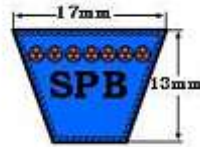
Figure 1.7: Designed V-belt section
